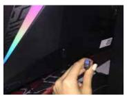
2. Using the OSD control button on the monitor, navigate to the Setup Menu and turn "ELITE RGB" on. Now you are ready to download the software.
